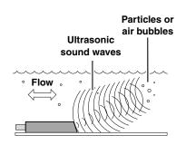
The 2150EX measures liquid level and average stream velocity, and calculates the flow rate and total flow. The liquid level and velocity measurements are read from an attached Area Velocity (AV) Sensor that is placed in the flow stream. Flow rate calculations are performed internally using the measured parameters from the AV Sensor. Additionally, the 2150EX can measure its input voltage.
